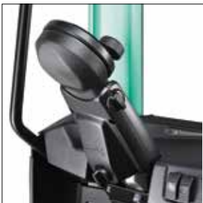
Folding steering wheel console
