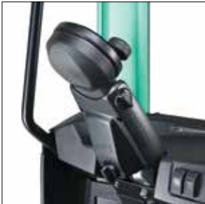
Folding steering wheel console
