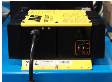
Figure 5: Default charge profile is displayed by the amber charging indicator light
