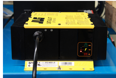
Figure 6: Red fault light blinking
